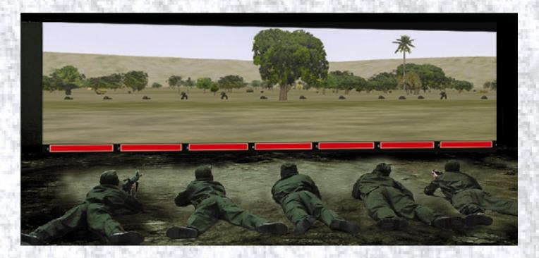
Advanced simulator for infantry shooting skill. From basic gunnery training to advanced shooting training programs. The gunners fire with invisible laser beam from the modified weapons to various types of targets on screen. The modified weapons produce simulated recoil force. Hit results are shown in many different ways giving immediate feedback and also after action review with reports.
